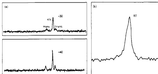
**Figure 1.** (a)  $^{19}\text{F}$  NMR spectra of *cis*- and *trans*- $\text{UO}_2\text{-(CF}_3\text{COCHCOCH}_3)_2\cdot(\text{CH}_3)_2\text{SO}$  obtained at  $-30$  and  $-40$   $^\circ\text{C}$  on a Varian 360-L spectrometer (60 MHz). (b) Spectrum at ambient temperature on a 90-MHz JEOL FX-900 instrument showing the *trans* compound as a shoulder on the side of the *cis* isomer.
